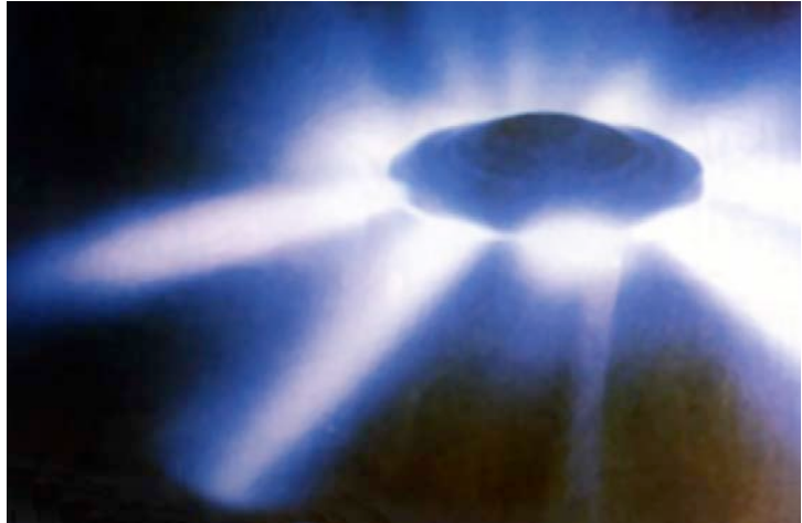
Figure 29. Picture of HF discharges. The sharp edge of this disk-shaped model made of an electrically conducting material makes radial HF discharges looking like “truncated light rays”.
